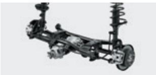
→ Rear chassis module Cross member, strut, axle, etc.
