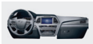
→ Cockpit module Airbag, audio/video, air conditioner/heater, cluster, glove box, etc.
