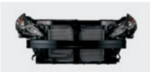
→ Front-end module Front-end's cooling module, head lamp, bumper, carrier, etc.
