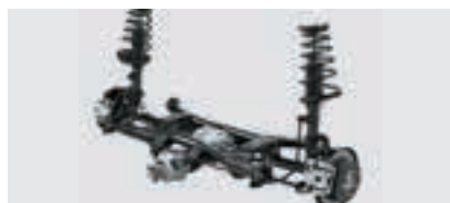
Rear chassis module Cross member, strut, axle, etc.
