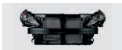
Front-end module Front-end's cooling module, head lamp, bumper, carrier, etc.
