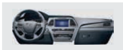
Cockpit module Airbag, audio/video, air conditioner/heater, cluster, glove box, etc.
