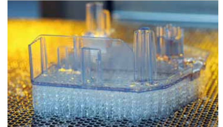
Test jig manufactured using the 3-dimensional printer
