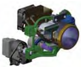
MOBIS' multi-function LED lighting system
