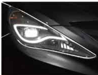
The pictured headlamp assembly consists of low beam, high beam, signal light, day time running lamp and side-marker lights. (Refer to the fuel use reduction and CO<sub>2</sub> emission reduction impact study published by the University of Michigan Transportation Research Institute for more details)
